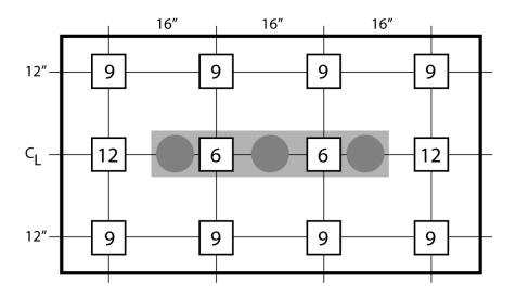
Discharge time in seconds (1000-100V) as shown are typical, fan speed set to high. Guardian blower 18" from CPM measuring plate. CPM test plate 1" from table. Discharge times slightly longer for 230 VAC, 50 Hz unit.
